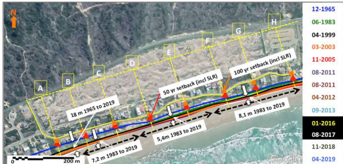
Figure 9: The position of the reference lines (A to H) and positions of the wave run-up line for the period 1965 to 2019 at Moquini Beach. The lines are superimposed at a common scale on the 2019 aerial image (Google Earth™)
